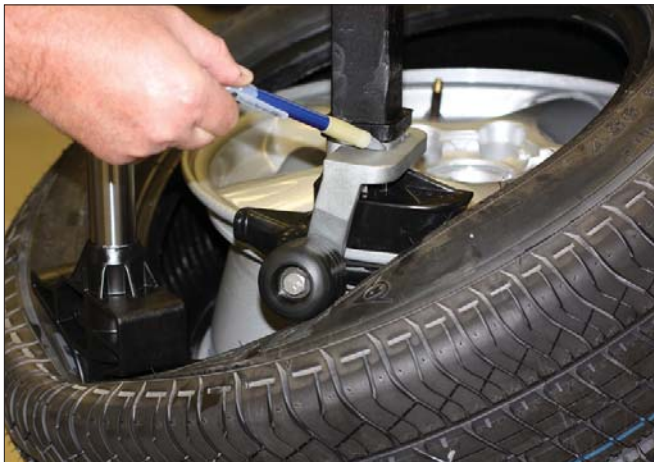
Figure 44 - Duckhead Roller Properly Mounted On Bracket
