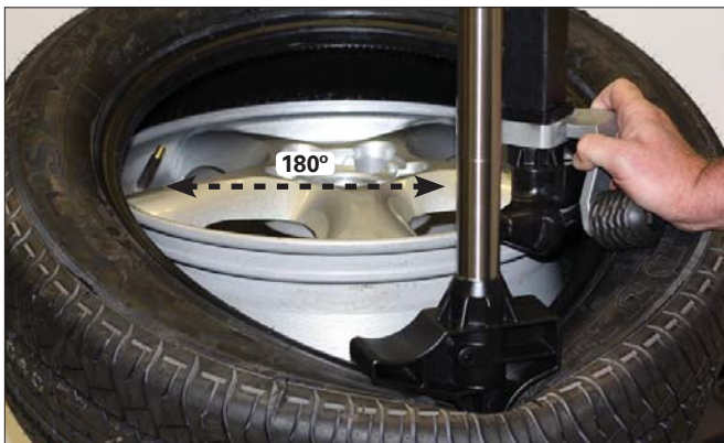
Figure 21 - Position Valve Stem 180° Ahead of Mount Tool
