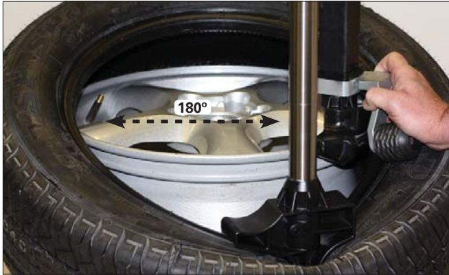
Figure 43 - Position Valve Stem 180° Ahead of Mount/Demount Tool
