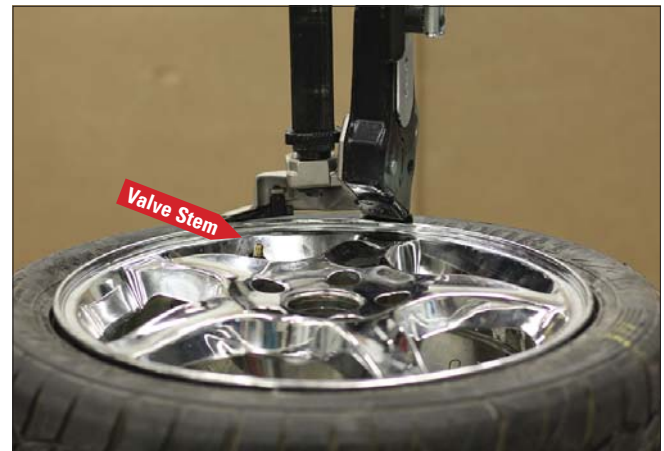
Figure 50 - Position Valve Stem Behind Leverless Demount Tool
