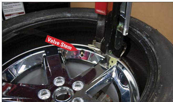
Figure 53 - Bead Lifter Tool Hooked Under Lower Tire Bead
