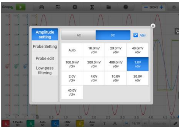
Figure 7-42 Amplitude Setting Screen (DC 1.0 V/div)
