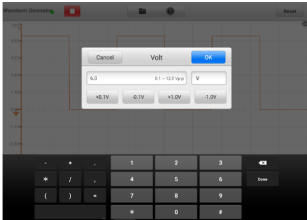
Figure 7-100 Voltage Setting Screen 3
