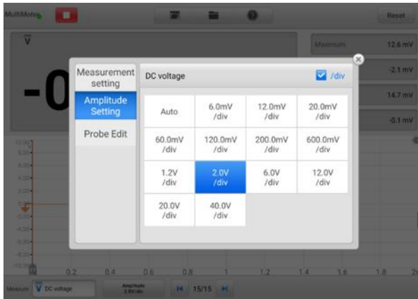
Figure 7-77 Amplitude Setting Screen (DC 2.0 V/div)
