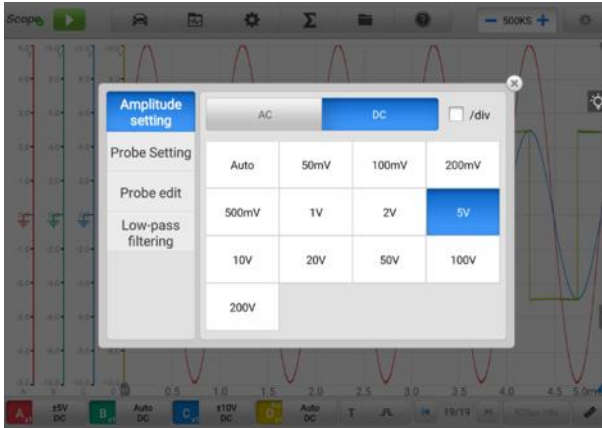
Figure 7-41 Amplitude Setting Screen (DC 5 V)
